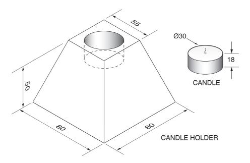
Draw a top view and sectioned front view of the candle holder in third angle projection. Do not draw the candle.
