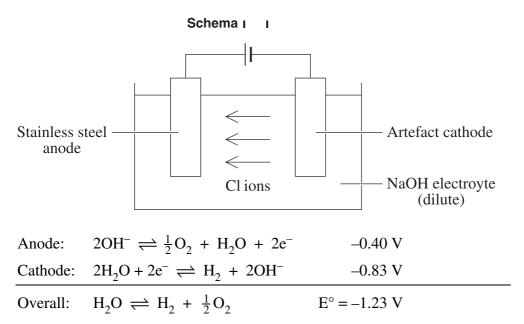
Knowledge of electrolysis is important to prevent damage to the artefact or hazards for conservators.
