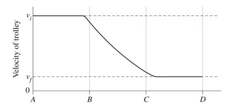
The velocity of the trolley is reduced as it passes through the region under the magnet (B) because its kinetic energy is transformed into heat energy in the copper plate.
