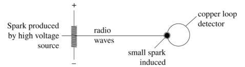
Further experiments using reflecting surfaces and other apparatus showed that radio waves can be reflected and refracted, behaviours consistent with visible light. A modification of the basic design allowed him to determine the velocity of the radio waves, using an interference pattern to determine their wavelength. Since the frequency was determined by the high voltage source, the wave equation  $v = f\lambda$  could be used. The value obtained was the speed of light.
