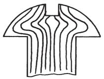
Candidates indicated that they were familiar with the concept of grainflow (they demonstrated that the grains flowed around the head of the bolt) and the notion that the slot had been machined.
