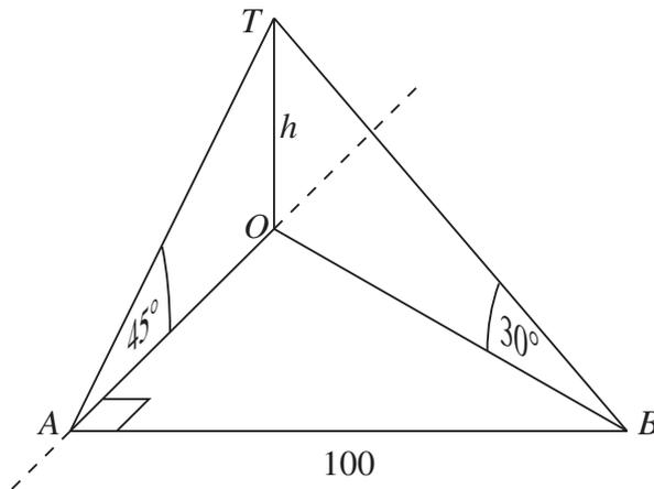
A surveyor stands at a point  $A$ , which is due south of a tower  $OT$  of height  $h$  m. The angle of elevation of the top of the tower from  $A$  is  $45^\circ$ . The surveyor then walks 100 m due east to point  $B$ , from where she measures the angle of elevation of the top of the tower to be  $30^\circ$ .
