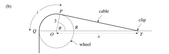
A long cable is wrapped over a wheel of radius 3 metres and one end is attached to a clip at T. The centre of the wheel is at O, and QR is a diameter. The point T lies on the line OR at a distance x metres from O.
