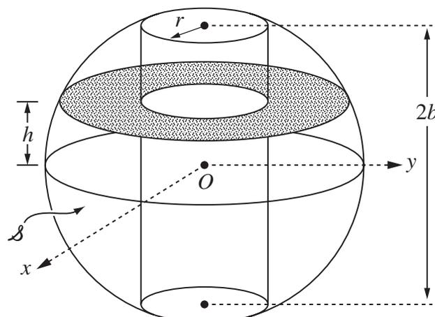
A cylindrical hole of radius  $r$  is bored through a sphere of radius  $R$ . The hole is perpendicular to the  $xy$  plane and its axis passes through the origin  $O$ , which is the centre of the sphere. The resulting solid is denoted by  $\mathcal{S}$ . The cross-section of  $\mathcal{S}$  shown in the diagram is distance  $h$  from the  $xy$  plane.
