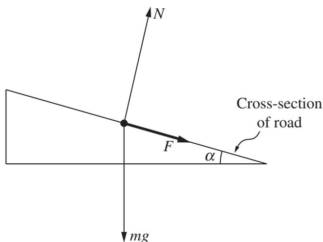
A road contains a bend that is part of a circle of radius  $r$ . At the bend, the road is banked at an angle  $\alpha$  to the horizontal. A car travels around the bend at constant speed  $v$ . Assume that the car is represented by a point of mass  $m$ , and that the forces acting on the car are the gravitational force  $mg$ , a sideways friction force  $F$  (acting down the road as drawn) and a normal reaction  $N$  to the road.
