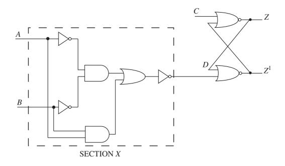
Identify the logic gate in SECTION X, and determine the state of Z and  $Z^1$  if input B changes to a value of 1. Use truth tables to justify your answer.
