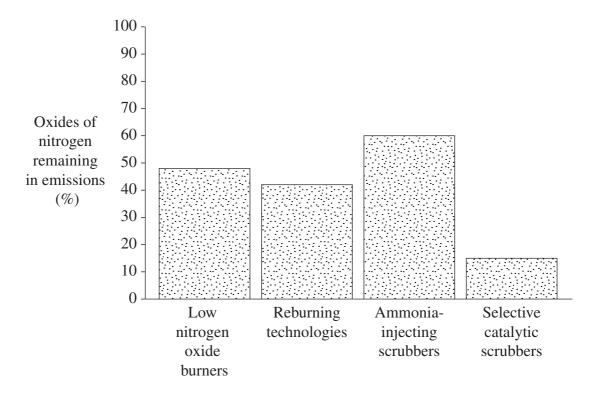
Which of the following is the most effective method for removing oxides of nitrogen produced by the combustion of coal?
