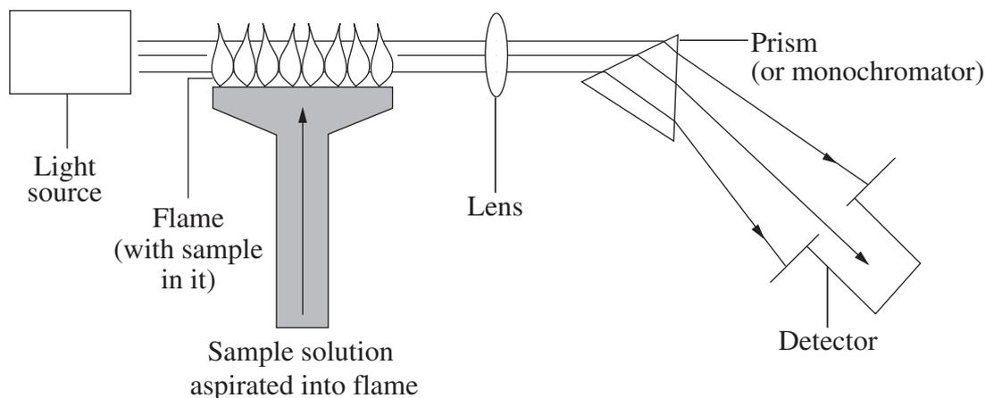
Principles – ground state (unexcited) atoms of an element irradiated by light of a particular wavelength will absorb light and become excited. By measuring the fraction of absorbed light, the concentration of the element in the sample solution can be determined.
