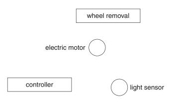
The block diagram is a graphical way for showing the relationships between the processors, controllers, censors and actuators – like a flow chart. It shows the processes and the devices involved, in a graphical format to make it easy to understand.
