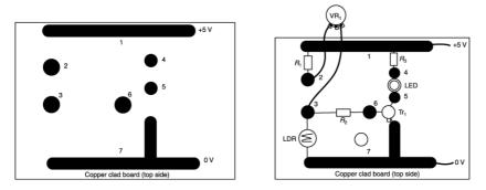
Issues to be considered in the design of the PCB track layout (mask):
