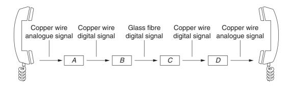
At what point does a conversion of electrical energy to light energy take place in this system?
