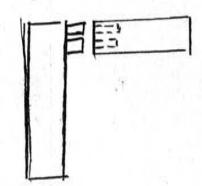
A donell joint could be used to construct the door with done held being drilled before they are nested. Glue can then be applied to the joint to hold it bosether.
