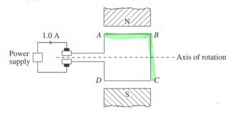
(a) Determine the force acting on section <u>AB</u> and the force acting on section <u>BC</u> due to the magnetic field, when the loop is in the position shown.
