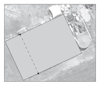
The width of the shed indicated by the dotted line was measured using an online ruler tool, and found to be approximately 12 metres.
