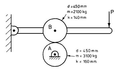
A force P is applied to bring the rollers together, so that a normal force of 20 kN is acting between the rollers.
