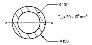
Determine the maximum tensile stress on the inner surface of the hollow beam due to bending at the wall.
