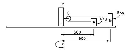
(a) Draw a free-body diagram of the forces acting on blocks *A* and *B* when they are on the point of sliding.
