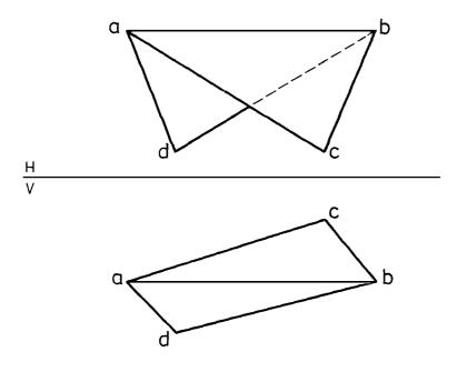
True angle between surfaces  $\ldots \ldots ^{\circ}$
