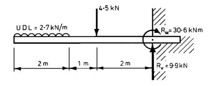
(i) Draw and fully label the shear-force diagram.
