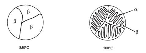
This question was poorly answered. Many candidates successfully sketched and labelled the 850°C structure but had little idea of the 500°C structure. Very few candidates identified the 500°C structure as a Widmanstatten structure. The most common responses were equiaxed grains of  $\alpha$  and  $\beta^1$  which demonstrated little understanding of the relationship between the two phases. Better candidates recognised that was a precipitate but often sketched it along the grain boundaries.
