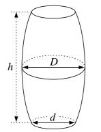
where *h* is the height of the barrel,*D* is the diameter at the centre of the barrel, and*d* is the diameter at the base of the barrel.
