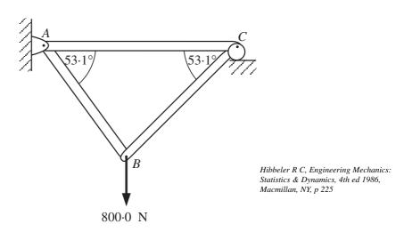
Member CA is horizontal. Each joint, A, B and C, is a pivot, and the joint C is free to move horizontally on the platform as shown. A load of  $800 \cdot 0$  N is applied vertically at pivot point B.
