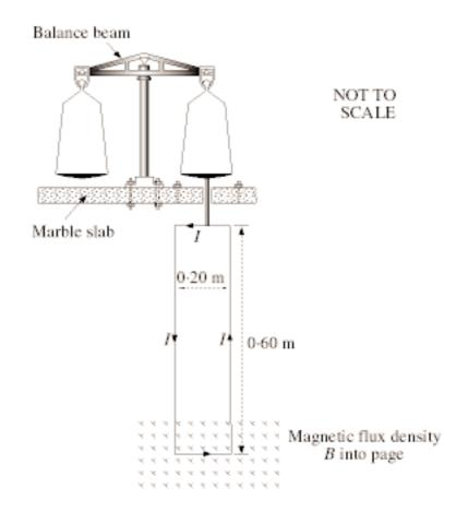
**30.** An apparatus, shown below, is designed to measure the magnetic flux density B of a magnet.
