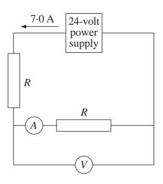
Assuming that both the ammeter and voltmeter are ideal, which pair of readings is correct?
