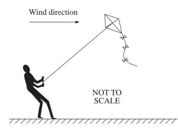
The forces acting on the kite can be resolved into four parts. These are the horizontal drag D, the weight W, the vertical lift L, and the force due to the tension in the string T. The mass of the kite is 0.40 kg.
