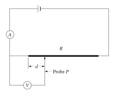
The resistor R is a length of resistance wire and the probe P is able to slide along the wire. The variable distance d of the probe P is measured from the left-hand end of R.
