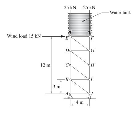
(a) (i) Calculate the magnitude of the vertical reactions at A and J, and the horizontal reaction at A.
