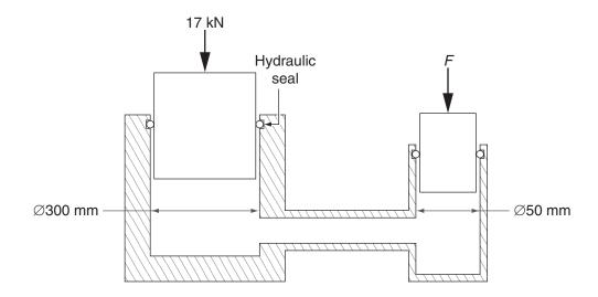
(i) Calculate the force (*F*) that must be applied at the small cylinder to lift a 17 kN load.
