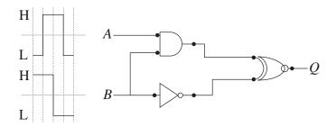
What is the resulting output waveform at Q?
