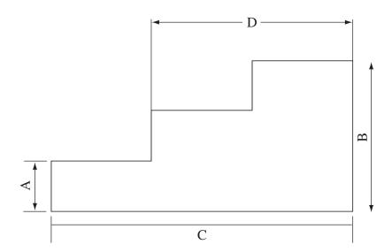
Which distance is correctly dimensioned?
