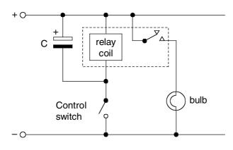
The capacitor needs to be in parallel with the relay coil.
