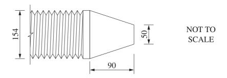
At which of the following angles will the compound slide need to be set, in order to produce the taper?
