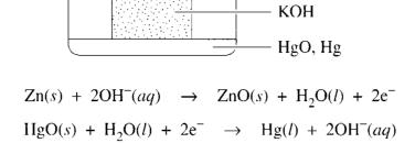
Identify the anode, cathode and electrolyte for this cell.
