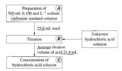
Describe steps **A**, **B** and **C** including correct techniques, equipment and appropriate calculations. Determine the concentration of the hydrochloric acid.
