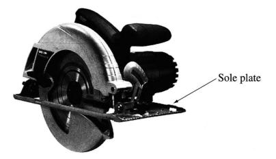
What are TWO adjustments that can be made to the sole plate? 2 (a) · Adjustments include the horizontal cutting angle which will allow for angled cuts of the hmber Also the plate can be adjusted to allow for <u>different</u> states the thickness of timber What features of the blade should be considered when purchasing a replacement? (b) 2 Features of the blade include the size or diameter of the place, aswell as the blade type or purpose, Eg Soft wood or hard wood cutting
