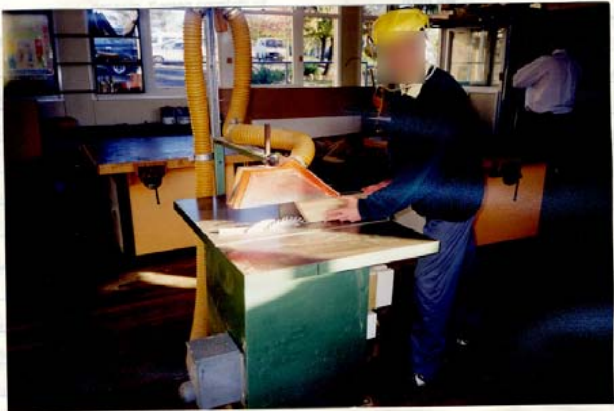
↑ Me using electric circular saw to get rough grain out of wood
