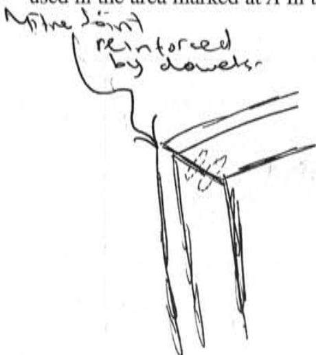
Mitre Joint - This is a common framing joint that is when two ends of the timber are cut at  $45^\circ$  to create a  $90^\circ$  angle. Can be reinforced by dowels or biscuits.
