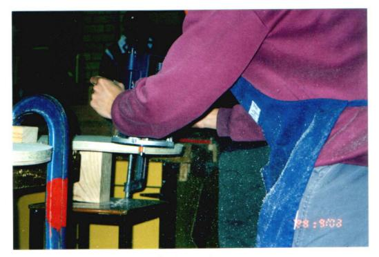
\* Notice the bearing follow the template underneath the particle board.
