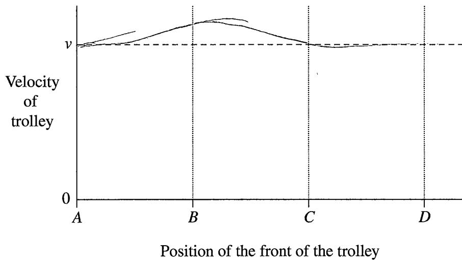
The trolley would speed up as it reaches the magnet and then slow down again as it has passed the magnet.
