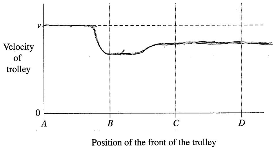
The copper plate is attracted to the strong magnet so it starts slowing down a bit after point A. Once it is past the magnet it then starts moving again but never reaches the initial velocity unless an external force increases. This is due to the magnet slowing the trolley down and the flat force prevents the initial velocity being reached.
