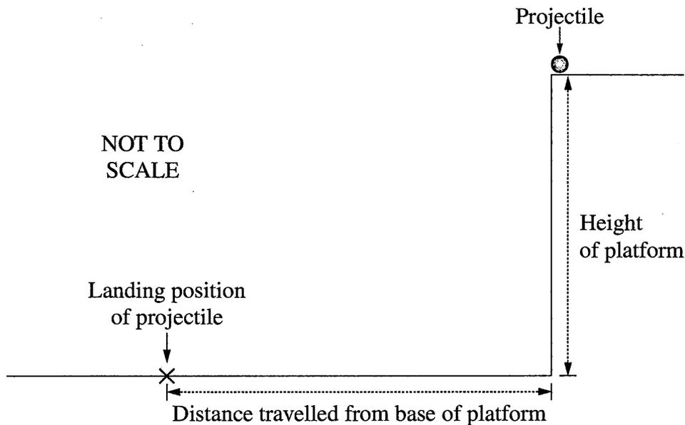
Measurements of the distance travelled by the projectile from the base of the platform are made for a range of initial velocities.
