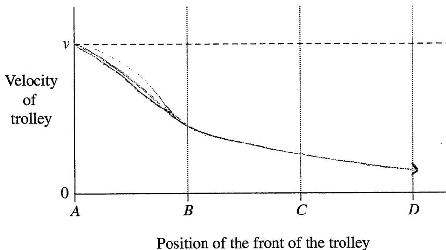
As the trolley moves towards (B), it sees a change in flux. This will cause eddy currents to flow (solid device) in a way that opposes the changing flux. This will cause the repel from the magnet & slow down. Due to its momentum however, it will move past (B) where the magnetic flux is now becoming smaller (thus changing) and the eddy currents will move in a way to
