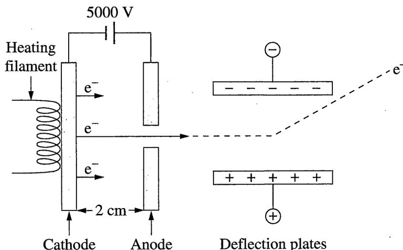
Electrons leave the cathode and are accelerated towards the anode.
