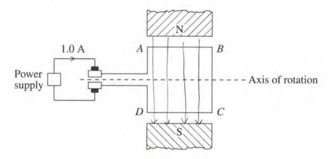
(a) Determine the force acting on section AB and the force acting on section BC due to the magnetic field, when the loop is in the position shown.
