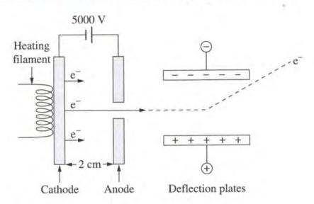
Electrons leave the cathode and are accelerated towards the anode.
