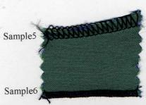
On the top of the train, where it drapes down from back shoulders, I experimented with a thicker, 4 reel thread overlock (sample?) compared to the previous 3 reel
